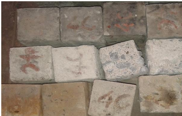
Fig.3 Specimens After Curing in Solutions
