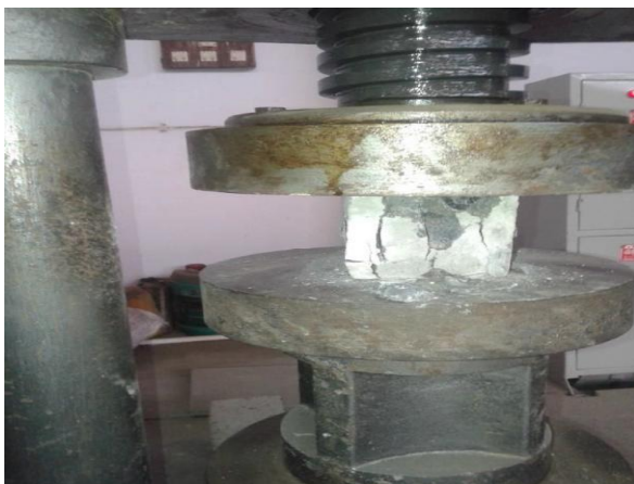
Fig.4 Testing of Specimen After Curing in Compression Testing Machine
