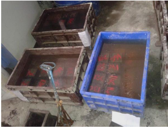
Fig.2 Specimens Exposed to H 2 SO 4 & HCl Solutions
