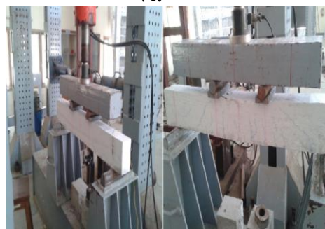
Fig 5: Two-Point Loading Setup & Crack Pattern identification
