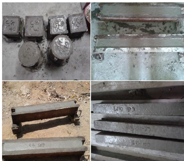
Fig 3: Casting of Cubes, Beam, Curing and remolding of beam
