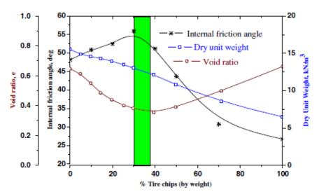
(Fig No.7 Internal friction angle, dry unit weight and void ratio profile with % TC)
