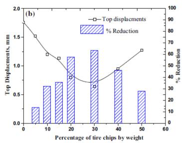
(Fig No.3 Displacement profile with different STC mixtures)
