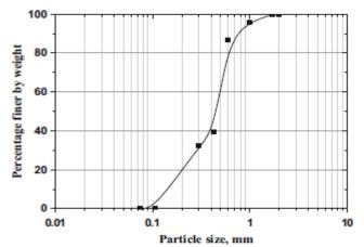
Figure 1.(Grain size distribution of the sand) Table No. 2- Properties of Sand
