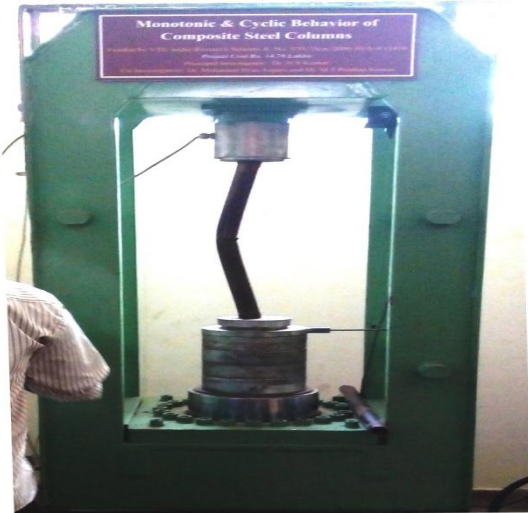
Fig 3: Monotonic Testing in UTM (R&D Lab, Department of civil engineering GCE, Ramanagaram)
