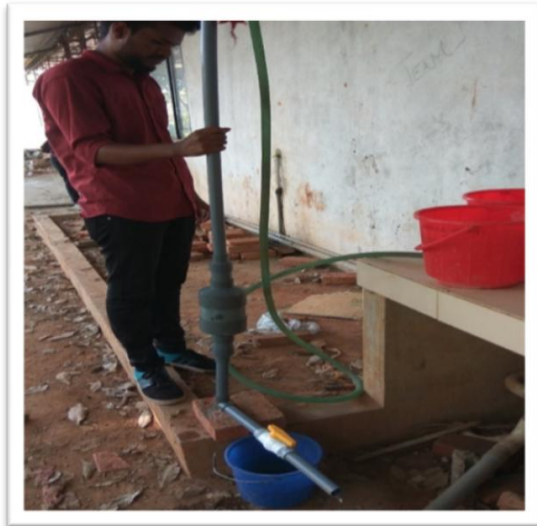
Fig. 5: Constant Head Permeability Test
