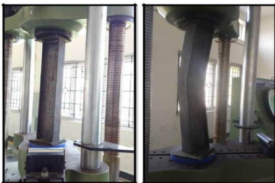
Fig 2: Fabrication, Testing and Buckling of I – section
