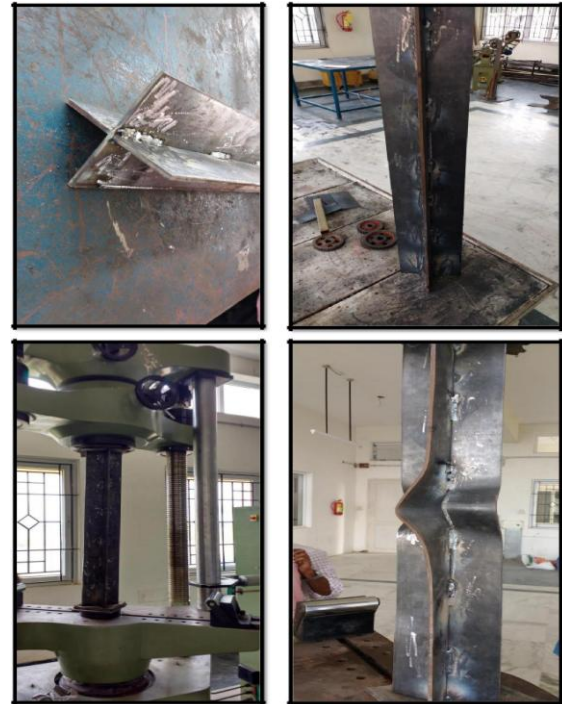
Fig 3: Fabrication, Testing and Buckling of Cruciform
