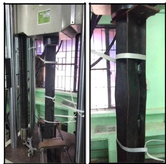
Fig 4: Fabrication, Testing and Buckling of Modified Cruciform
