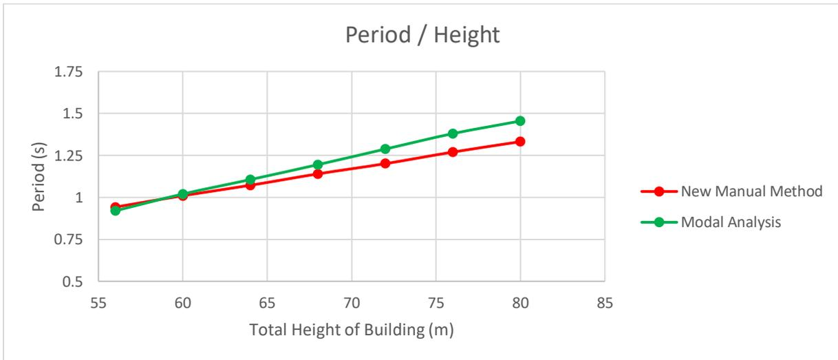
**Fig.16 Period-Height Graphs for New Manual Method and Computer Analysis (Modal Analysis)**
