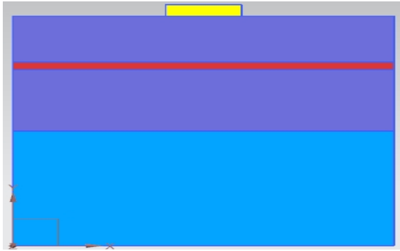
Figure 5.8 FEM Model of foundation with geogrid at u= 300mm
