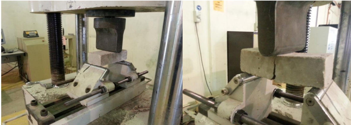
Fig. 4: Flexural Strength Test on Bricks
