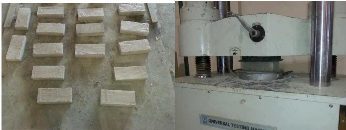
Fig. 3: Brick Specimen and Compressive Strength Test
