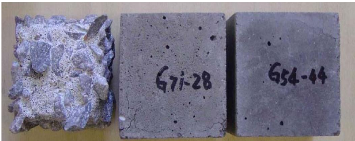
Fig. 6. Conventional concrete and Geopolymer concrete specimens (G71-28 & G54-44) after sulfate attack (X. J. Song et al. 2005)
