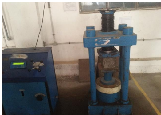
Fig 4 Cube compression test
