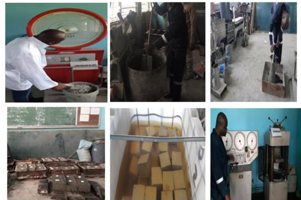
Plate 1: process photographs for Batching, mixing, slump, labelling, curing and crushing.
