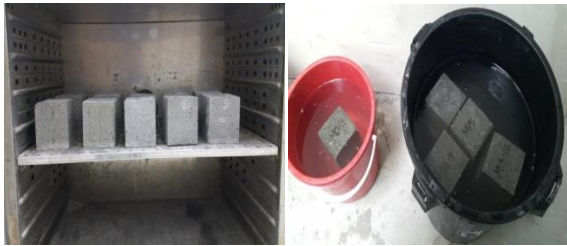
(a) Drying of mortar cube in oven (b) Immersion of mortar cube in water
