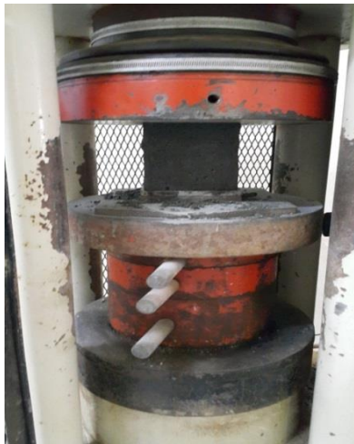
Fig 2: Mortar cube specimen under compressive axial load
