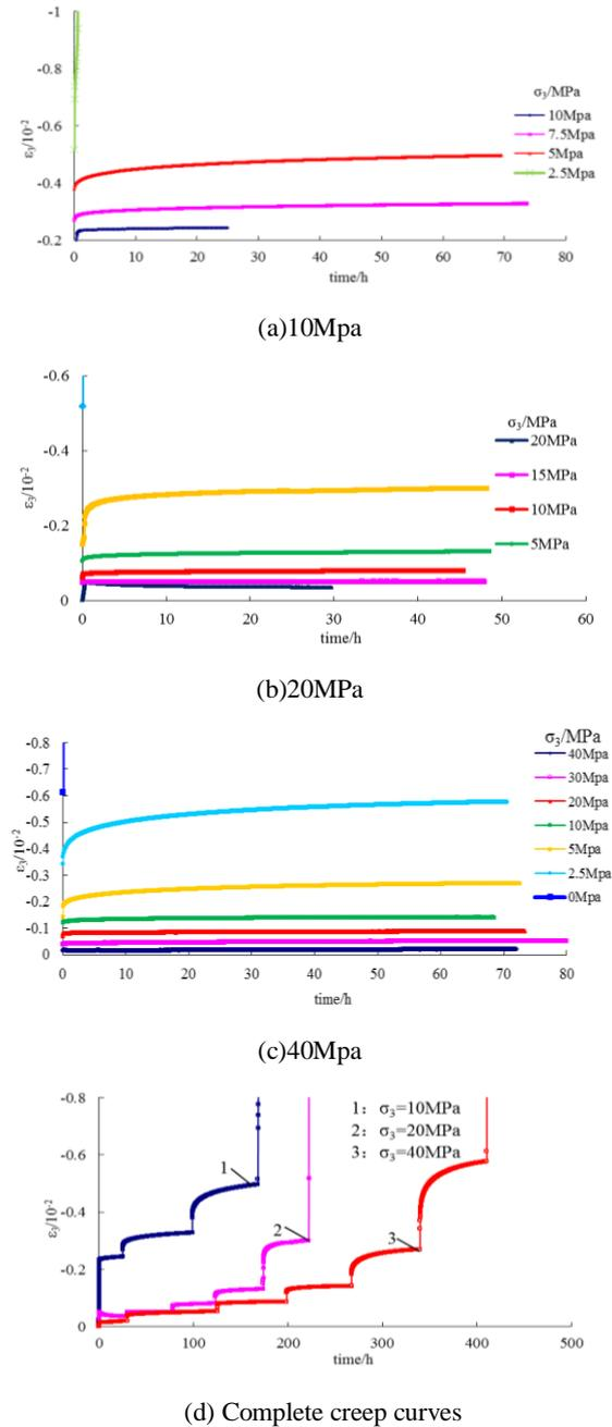
**Fig 4: Lateral creep curves under various unloading confining pressure**
