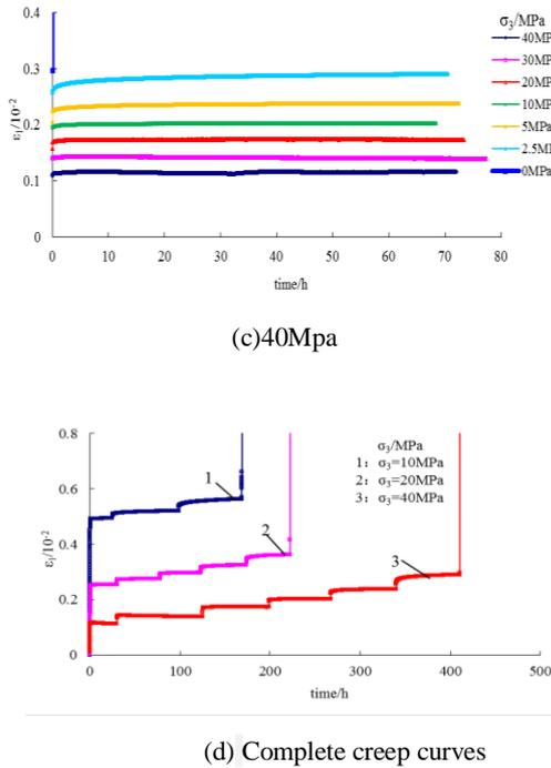
**Fig 3: Axial creep curves under various initial unloading confining pressure**
