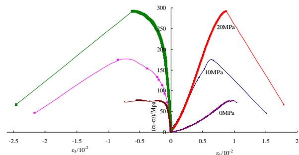
**Fig 2: Stress-strain curves of granite specimens under different confining pressure**
