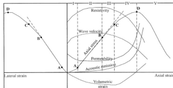
**Fig 7: Curves of physical and mechanical characteristics of rock specimens in triaxial compression tests**
