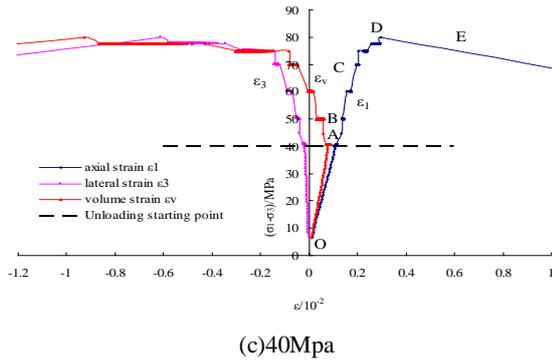
**Fig 6: Creep stress-strain curve under various CP**
