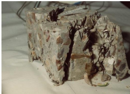
Fig. (04)compression failure mode for a concrete amorphousfibers Source 5
