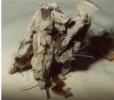
Fig. (03)compression failure mode for Concretehook fibers. Source 5
