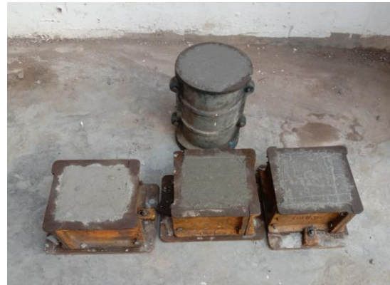
Fig 1: Casting of Cubes
