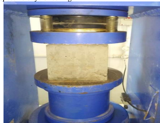
Fig 3: Compression test on Cubes
