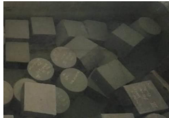
Fig 2: Curing of Cubes
