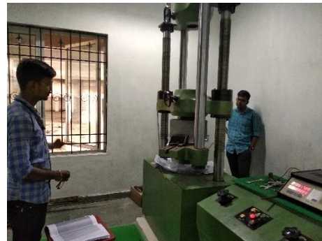
Fig 10: Compression test on blocks
