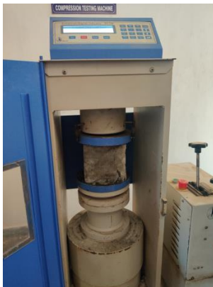
Fig.5 Compression test on concrete
