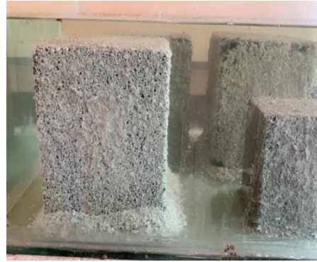
Fig.6 Acid Attack on Concrete
