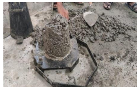
Fig.2 Slump Cone Test
