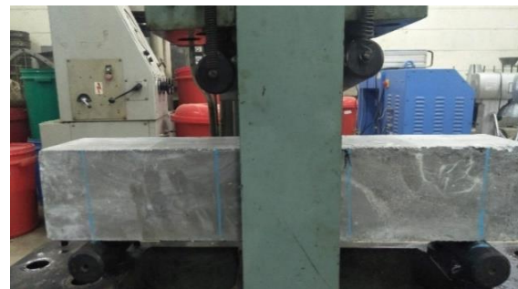
Fig. 2: Concrete Prism on Testing Machine
