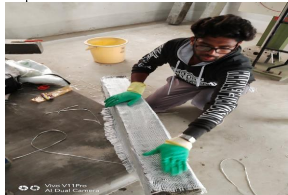
Figure-2 Glass Fiber wrapping on Beam
