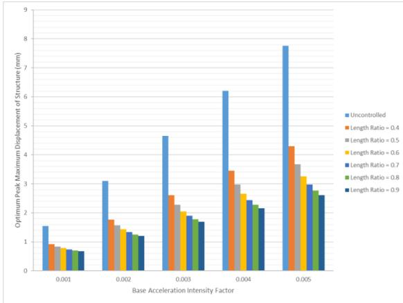
**Figure 8(a): Optimum Peak maximum Displacement of the structure for different length ratios and base acceleration intensity factors.**
