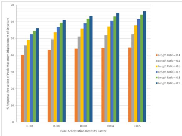
**Figure 8(b): Percentage response reduction of the maximum peak Displacement of the controlled structure with respect to the uncontrolled structure for various length ratios and base acceleration intensity factors.**
