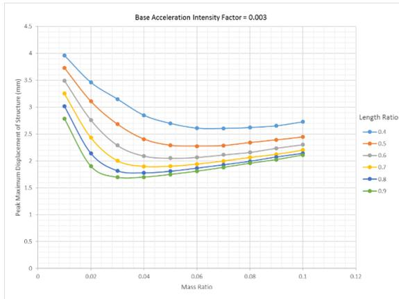
**Figure 6(b):** Peak maximum Displacement of the structure for various mass ratios and length ratios, corresponding to the base acceleration intensity factors of 0.003
