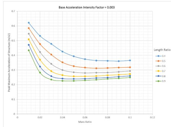
**Figure 7(b):** Peak maximum Acceleration of the structure for various mass ratios and length ratios, corresponding to the base acceleration intensity factors of 0.003
