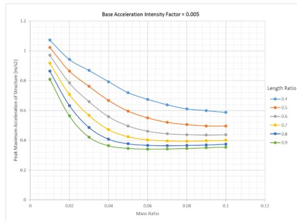
**Figure 7(c):** Peak maximum Acceleration of the structure for various mass ratios and length ratios, corresponding to the base acceleration intensity factors of 0.005
