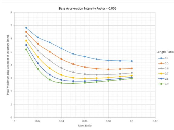
**Figure 6(c):** Peak maximum Displacement of the structure for various mass ratios and length ratios, corresponding to the base acceleration intensity factors of 0.005
