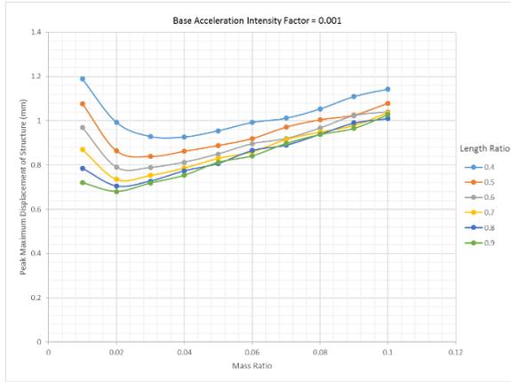
**Figure 6(a):** Peak maximum Displacement of the structure for various mass ratios and length ratios, corresponding to the base acceleration intensity factors of 0.001
