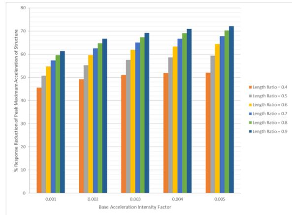
**Figure 9(b): Percentage response reduction of the peak maximum Acceleration of the controlled structure with respect to the uncontrolled structure, for various length ratios and base acceleration intensity factors.**
