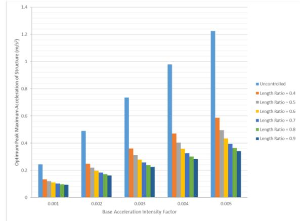
**Figure 9(a): Optimum Peak maximum Acceleration of the structure for different length ratios and base acceleration intensity factors.**
