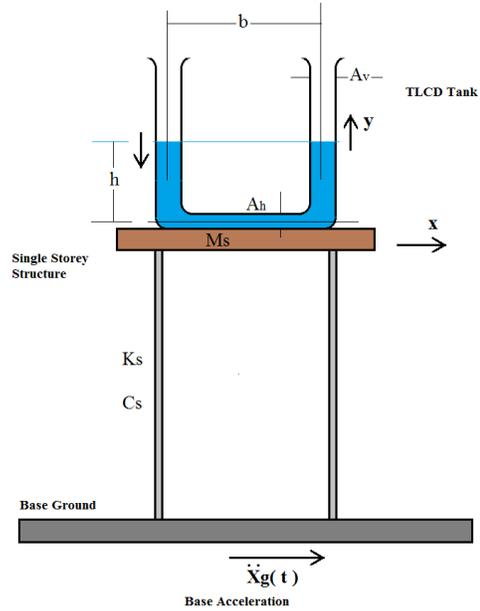
Figure. 1(a): Modeling of a single-story structure equipped with TLCD, idealized as SDOF system.
