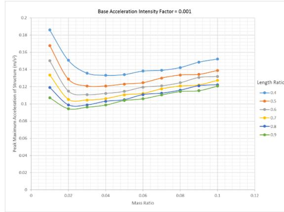
**Figure 7(a):** Peak maximum Acceleration of the structure for various mass ratios and length ratios, corresponding to the base acceleration intensity factors of 0.001
