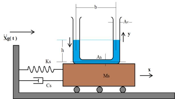
Figure. 1(b): An equivalent spring-mass system for SDOF structure system equipped with TLCD.
