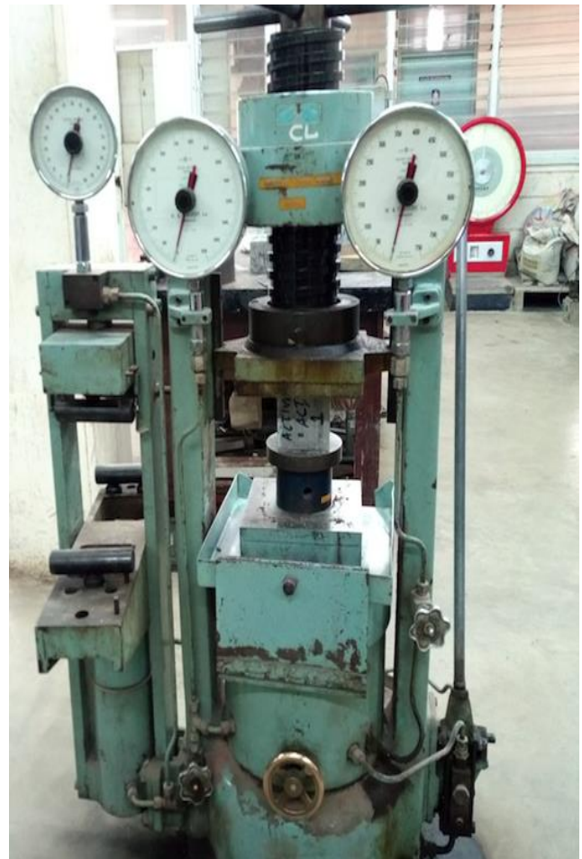
Fig. 4: Testing of compressive strength
