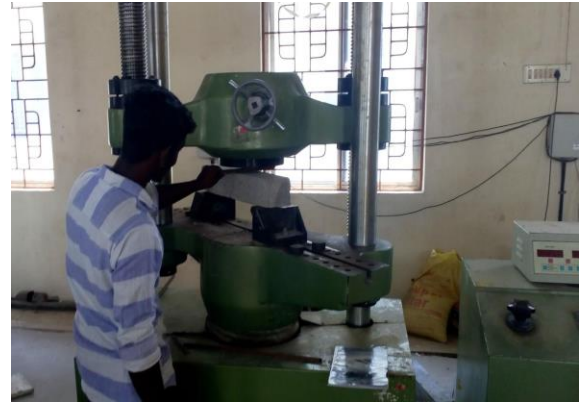
Fig.5 Flexural Test (Beam Strength)
