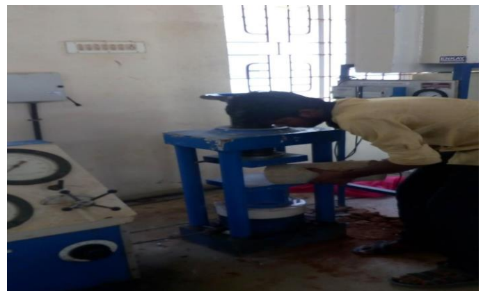
Fig.3 Split Tensile Test (Cylinder Strength)
