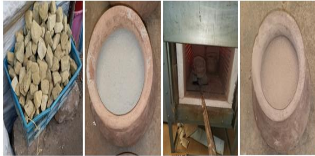
Fig 2: Transformation process of Kaolin in Metakaolin
