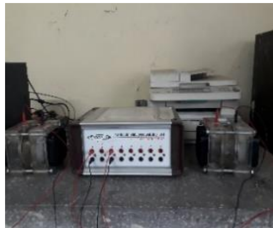
Fig.4 Rapid Chloride Permeability Test
