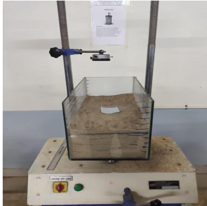
Fig. 1 GRS soil slope provided with reinforcement spacing
