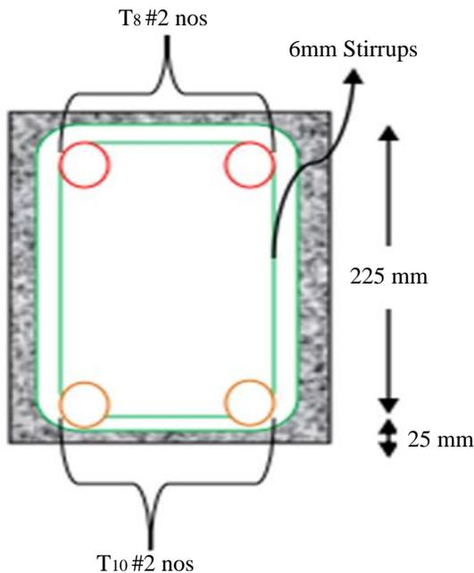
**Fig. 2 Cross section of the beam (all dimensions are in mm)**
