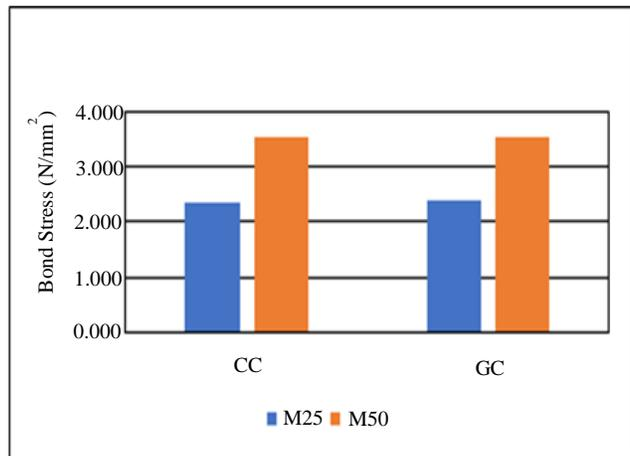
Fig. 18 Bond stress for HYSD bar
