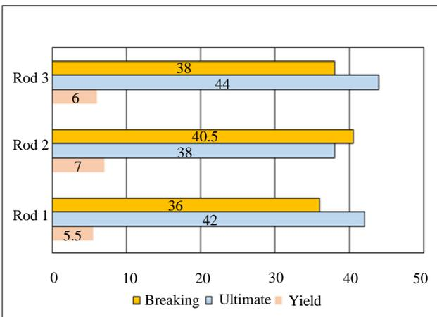
Fig. 15 Pull-out test for GFRP rod
