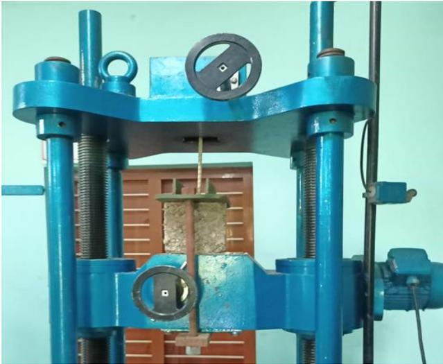
Fig. 6 Pull out test setup
