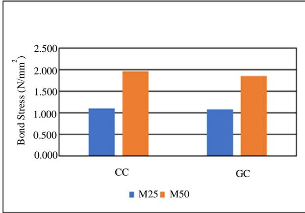
Fig. 19 Bond stress for GFRP bar
