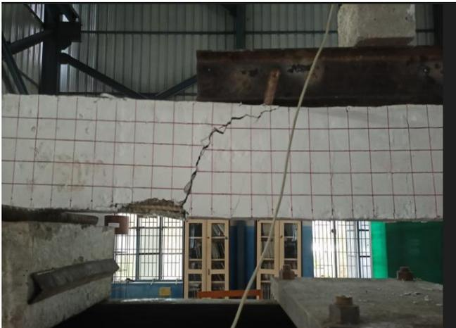
**Fig. 9 GFRP beam cracking stage**
