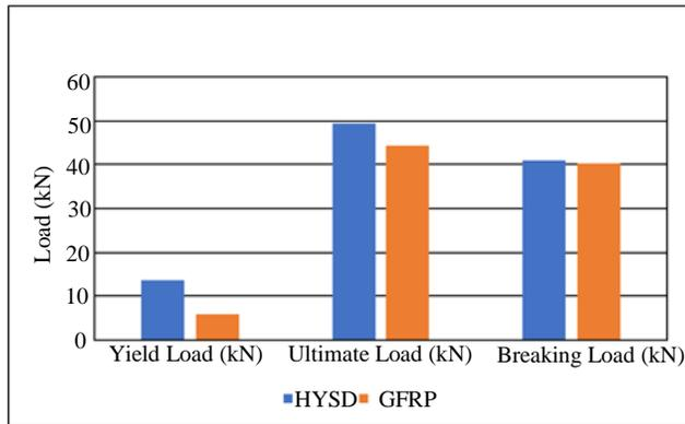
Fig. 20 Comparison of tensile test for HYSD and GFRP rod
