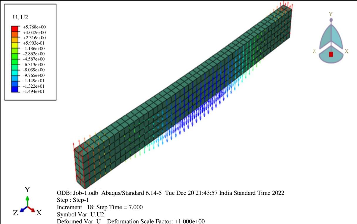
Fig. 3 Modelling of reinforcement deflection
