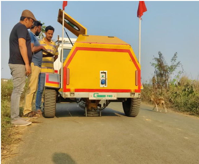
Fig. 9 FWD deflection recording on existing Jibantala-Taldi road
