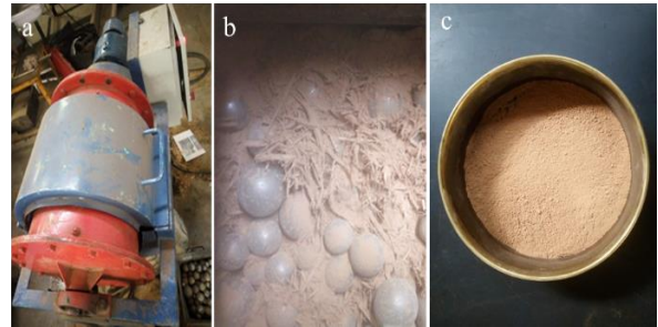
Fig. 1 Preparation of GBBP: (a) Ball mill used in the study, (b) Grinding of GBB, and (c) GBBP sieved through 105µm.
