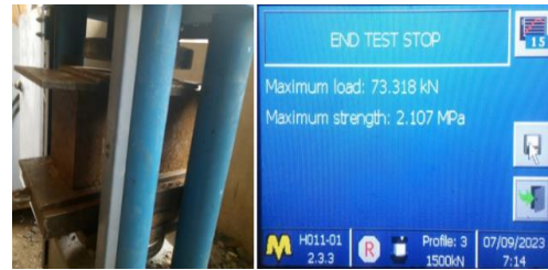
Fig. 2 Compressive strength set-up
