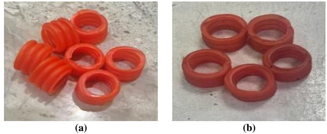
Fig. 7 Pieces of spiral electric hose (a) Before using it, and (b) After the operation period.
