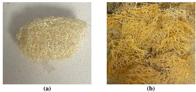
Fig. 10 Natural Loofah (a) Before using it, and (b) After the operation period.
