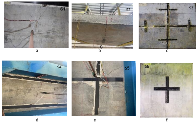
Fig. 9(a)-(f) First crack of all tested specimens
