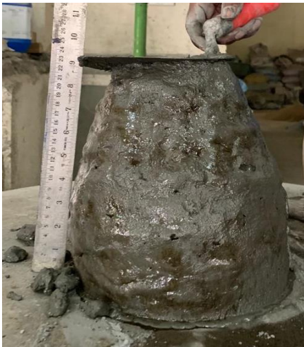
Fig. 4 Measured Slump of HSC
