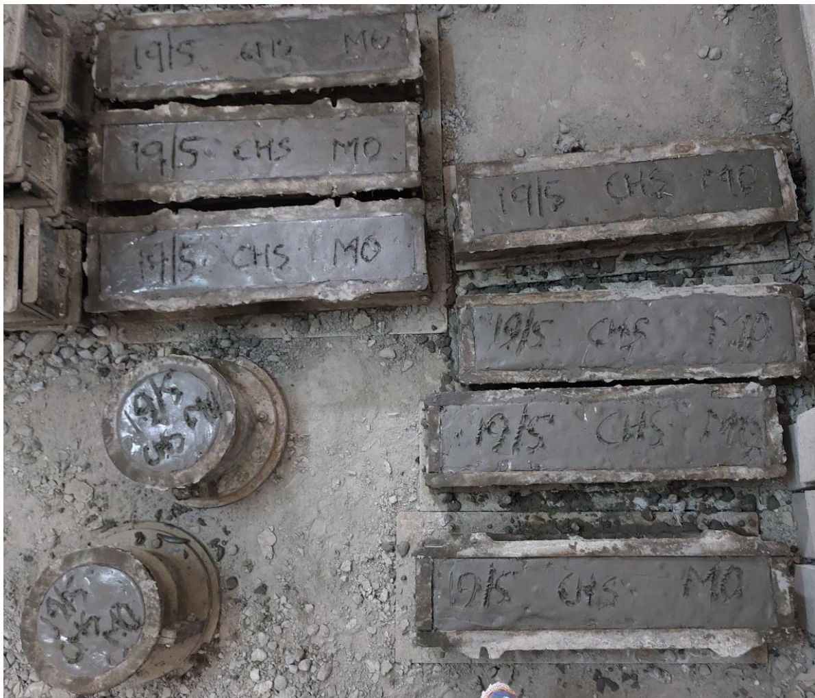
Fig. 5 Cylindrical and Prism specimens of HSC
