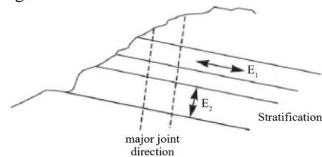
Fig. 14 Jointed rock model [16]
