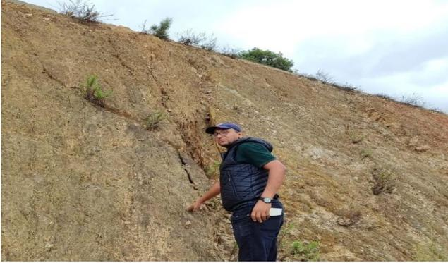
Fig. 8 Affected schist mass showing several marly joints
