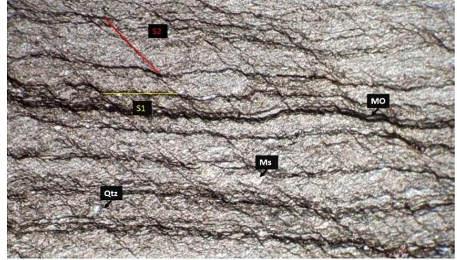
Fig. 9 Photographs of thin sections: S2 foliation with white micas (muscovite), quartz (qtz), and opaque minerals (observed in polarizing light microscopy)
