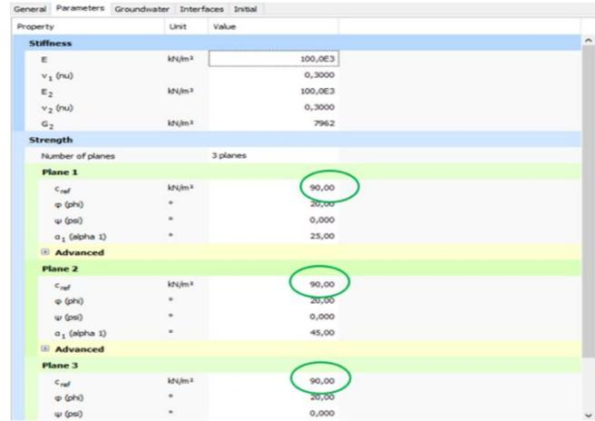
Fig. 18 Calculation model selected according to multiple planes, section N° 10
