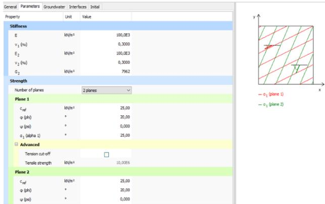
Fig. 16 Calculation model selected based on two planes, section 10
