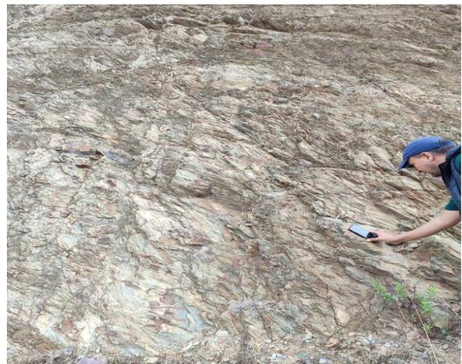
Fig. 7 Flaky structure of schists affected by an intense fracturing network
