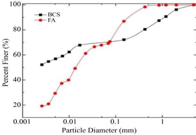
Fig. 3 Analysis of grain size-black cotton soil and fly ash
