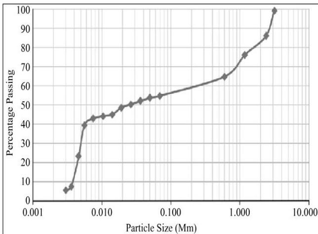
Fig. 2 Grain size analysis of BC soil
