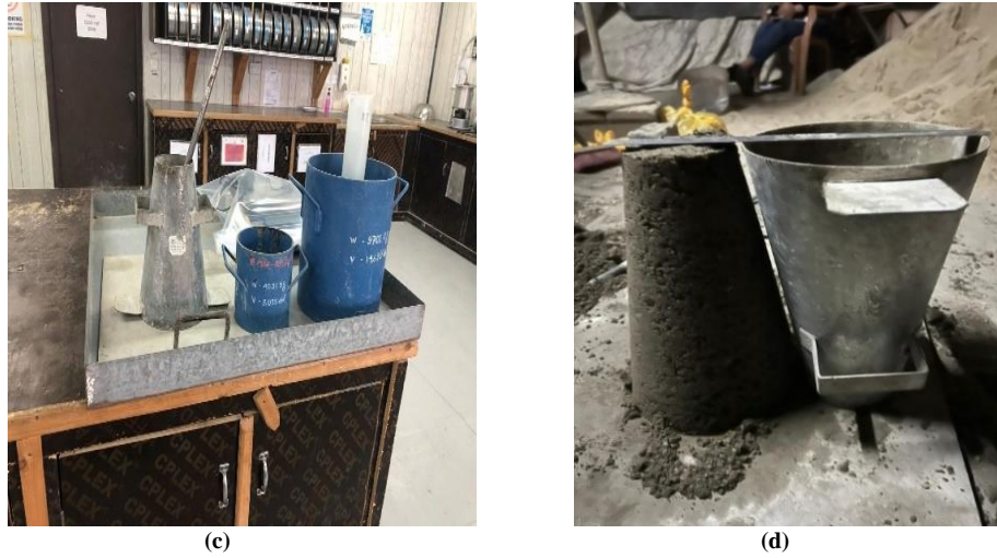
Fig. 6 (a) Measuring the amount of water, (b) Mixing of Constituent Materials, (c) Measuring apparatus, and (d) Slump test
