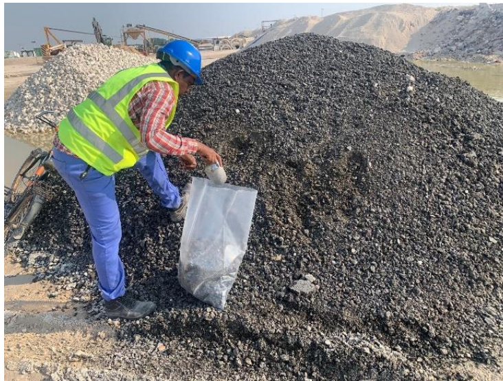
Fig. 4 Stockpile of Reclaimed Asphalt Pavement (RAP) at construction site
