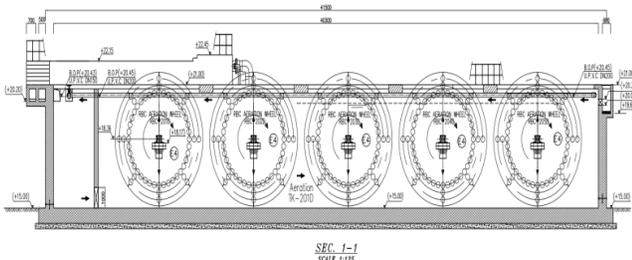
Fig. 7 Cross-section of the Biological Tank
