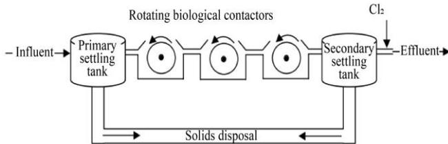
Fig. 1 Flow diagram of an RBC process[2]
