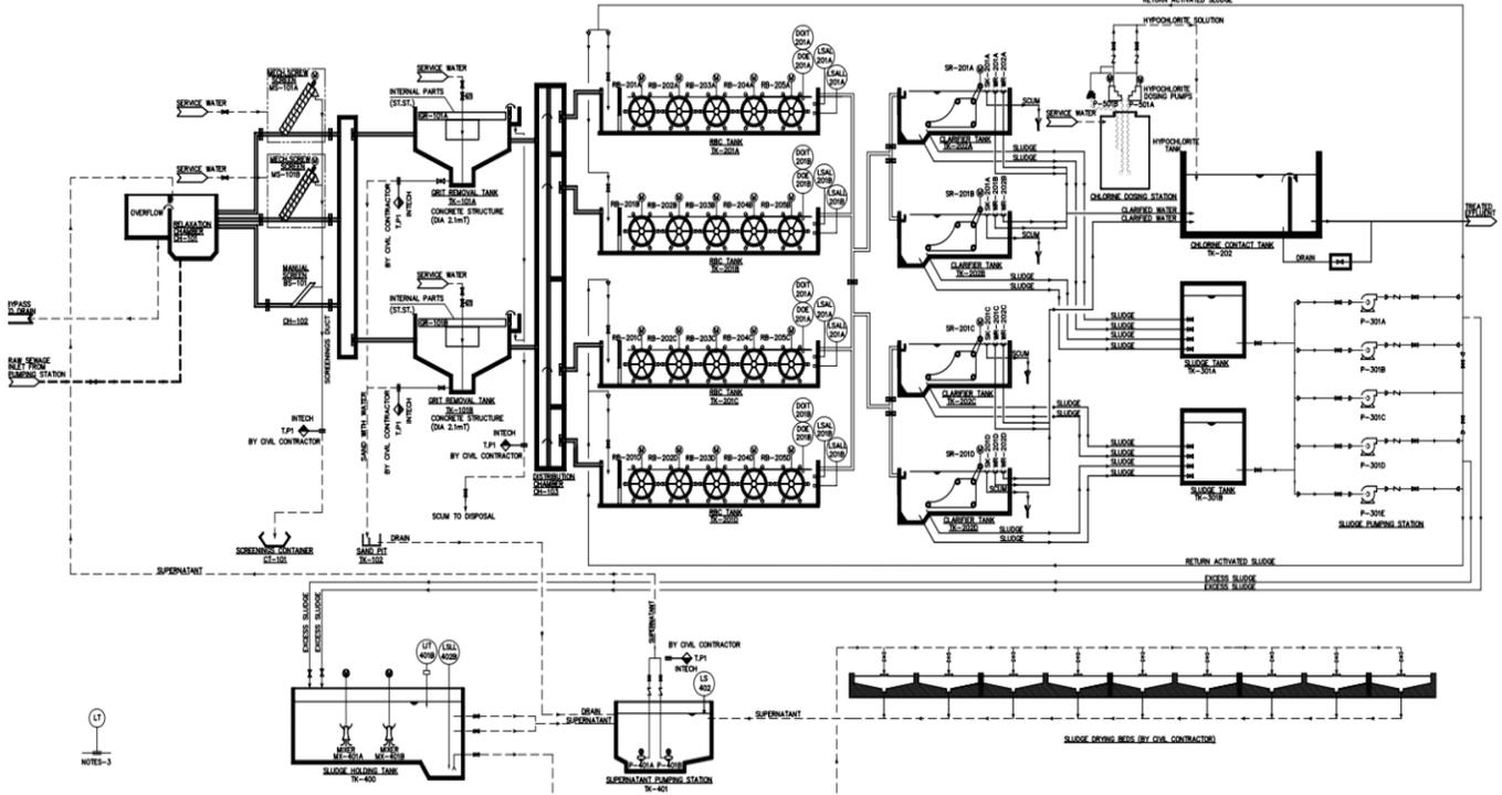
Fig. 6 El-Manayel WWTP process flow diagram
