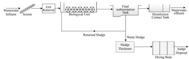
Fig. 3 Flow Diagram for El-Manayel WWTP
