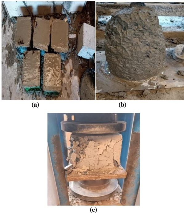
Fig. 4 Pictorial representation of: (a) Casting of cubes, (b) Slump test, and (c) Compressive strength test
