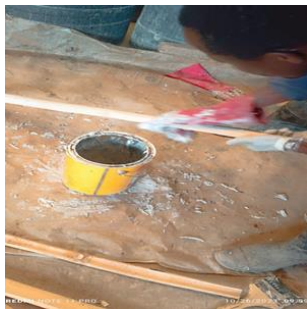
Fig. 2 Coating bamboo bars using Sikadur 32
