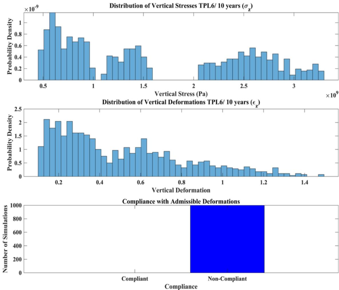
Fig. 18 Distributions of Vertical Stresses and Deformations TPL6/ 10 years and the compliance with admissible deformations
