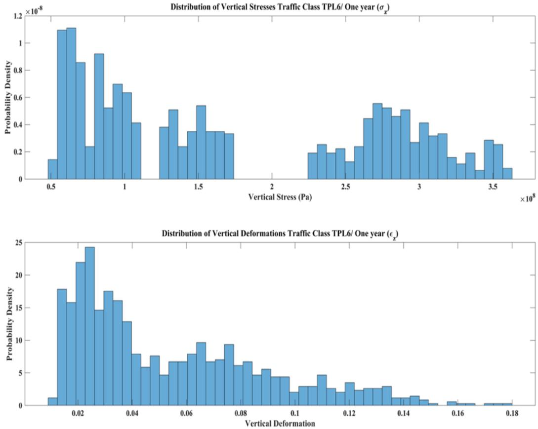
Fig. 11 Distributions of Vertical Stresses and Deformations for Traffic Class TPL6/ One year
