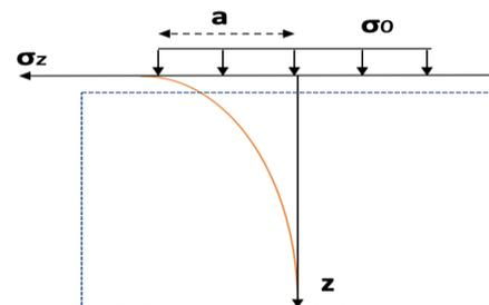
Fig. 2 Modeling of the surface load applied by the passage of a heavy truck wheel
