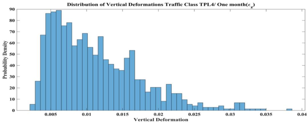
Fig.4 Distributions of Vertical Stresses and Deformations for Traffic Class TPL4/ One month
