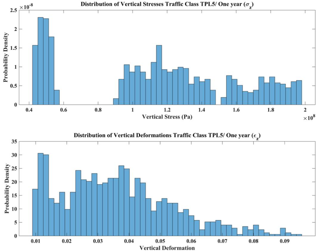
Fig. 8 Distributions of Vertical Stresses and Deformations for Traffic Class TPL5/ One year
