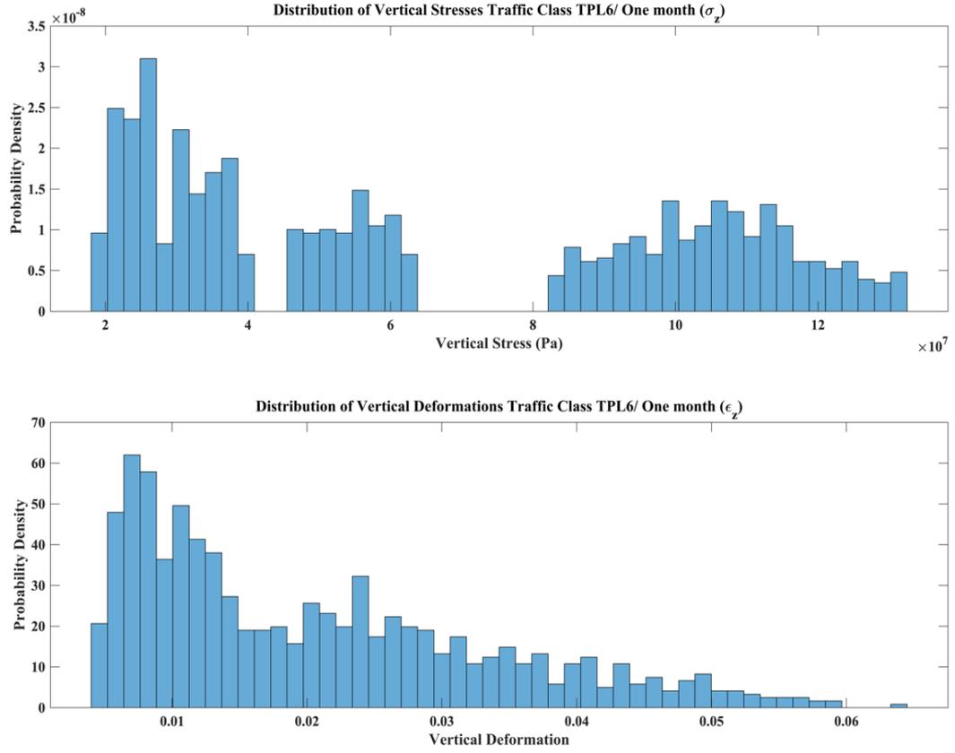
Fig. 10 Distributions of Vertical Stresses and Deformations for Traffic Class TPL6/ One month
