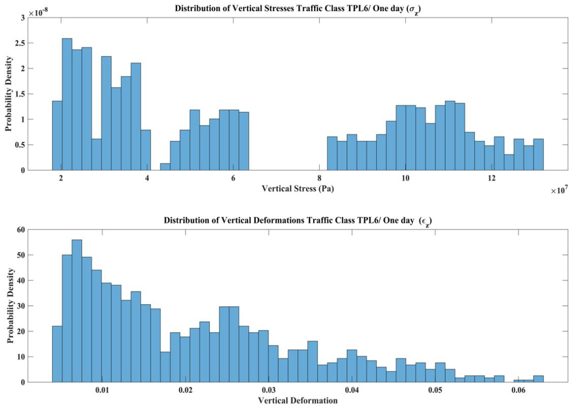
Fig. 9 Distributions of Vertical Stresses and Deformations for Traffic Class TPL6/One-day
