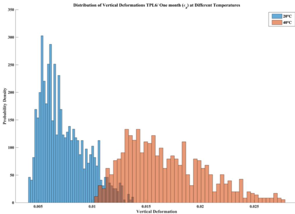
Fig. 20 Distribution of Vertical Deformations Traffic Class TPL6/ One month at different temperatures
