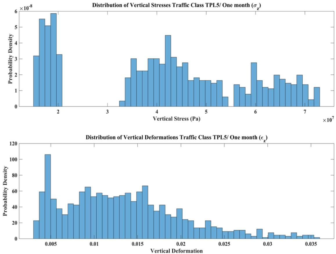
Fig. 7 Distributions of Vertical Stresses and Deformations for Traffic Class TPL5/ One month
