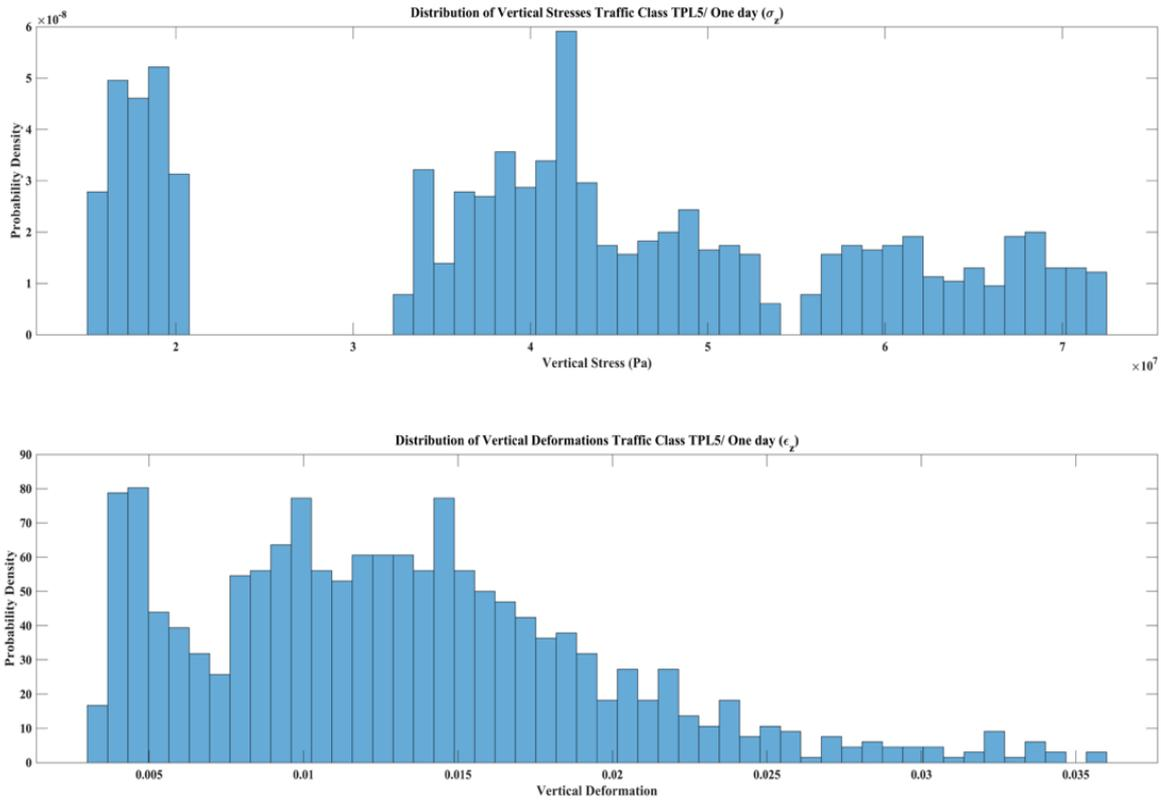
Fig. 6 Distributions of Vertical Stresses and Deformations for Traffic Class TPL5/One-day
