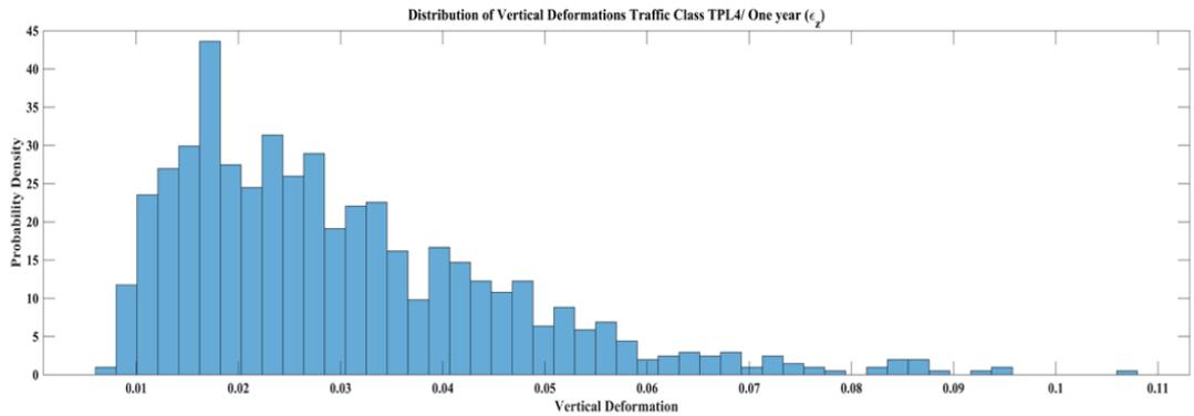
Fig. 5 Distributions of Vertical Stresses and Deformations for Traffic Class TPL4/One-year
