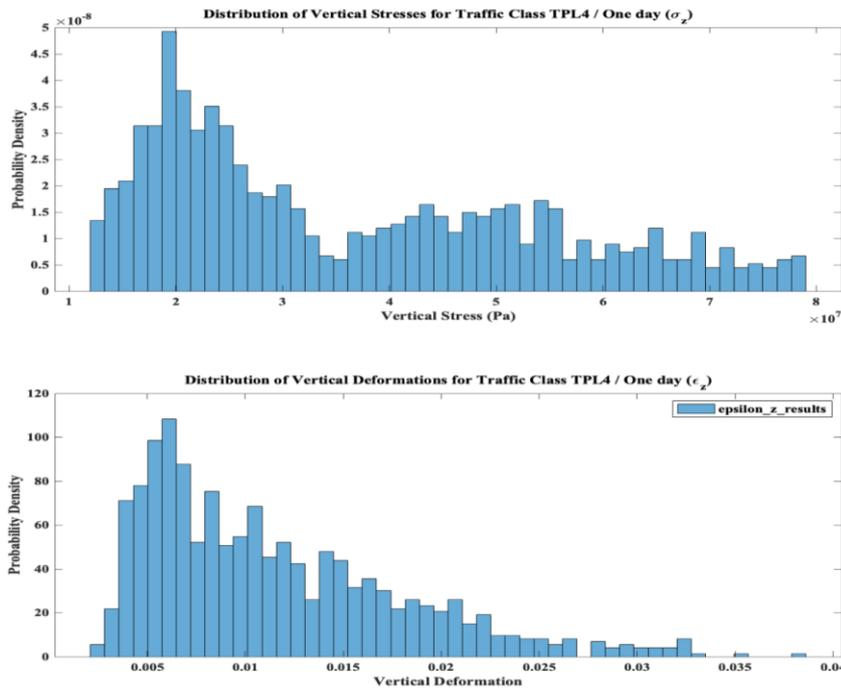
Fig. 3 Distributions of Vertical Stresses and Deformations for Traffic Class TPL4/One-day
