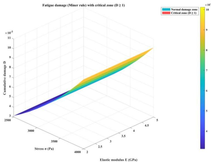
Fig. 17 Fatigue damage with critical zone
