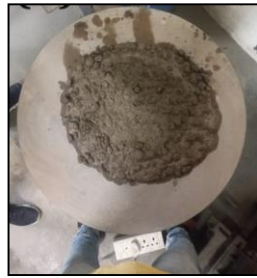
(b) Flow Table test
