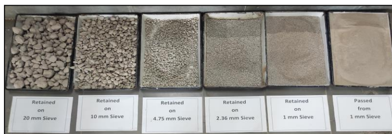
Fig. 2 Recycled CDW transformed into varying particle size
