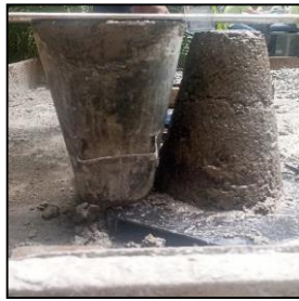
(a) Slump test
