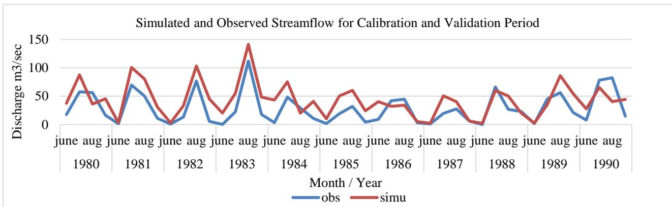
Fig. 5 Observation and simulation of discharge for Chaskaman station
