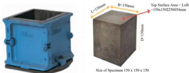
Fig. 3 Cube casting moulds and standard size of the cube
