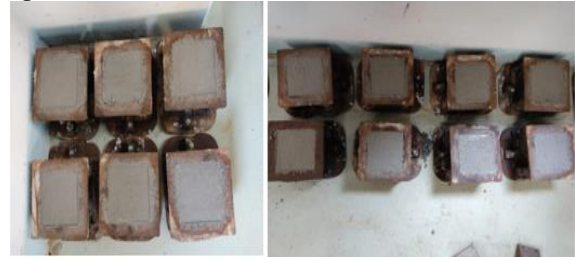
Fig. 4 Casting of concrete moulds
