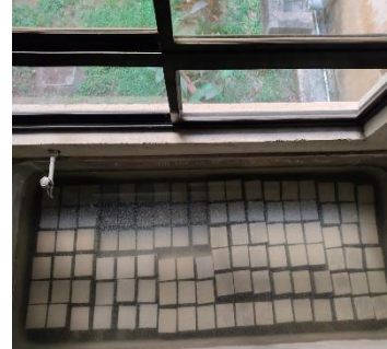
Fig. 5 Curing of concrete cubes
