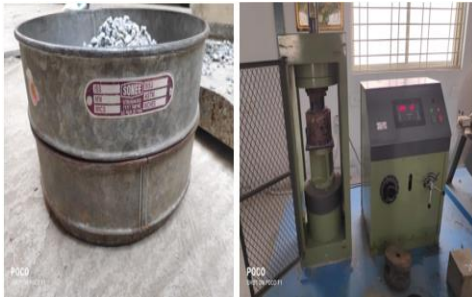
Fig. 2 Crushing test mould, sieves used and crushing test machine
