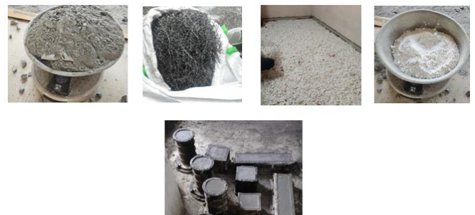
Fig. 5 Stages of concrete specimen preparation
