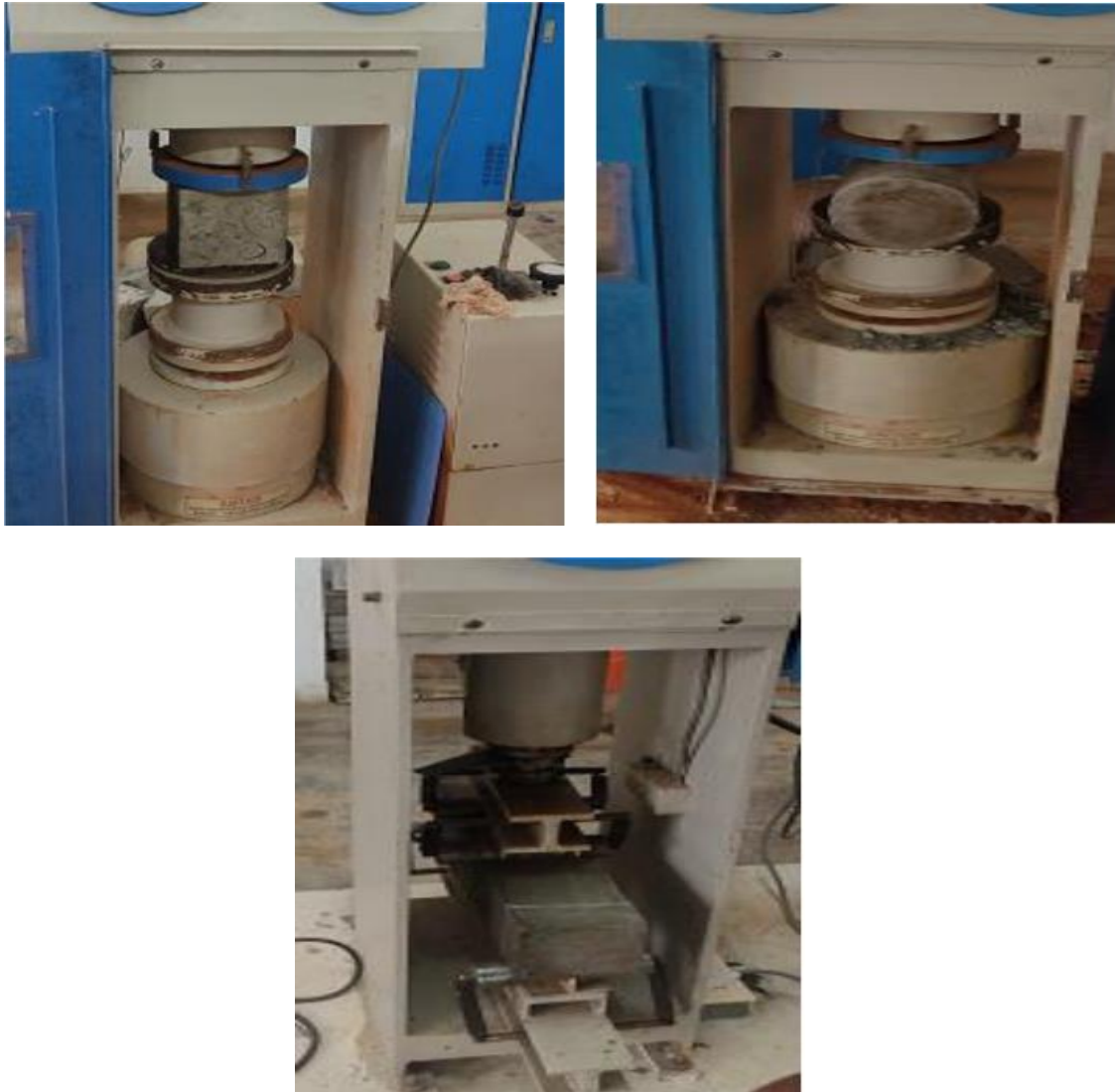
Fig. 6 Testing concrete specimens
