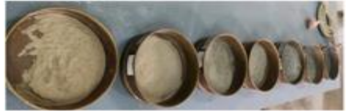
Fig. 2 Sieve analysis setup
