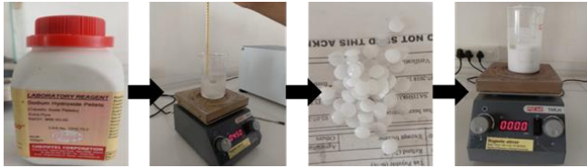
Fig. 1 Preparation of nano lime using the Sol-gel technique
