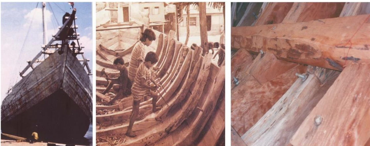
Fig. 1 Pinisi ship joint system
