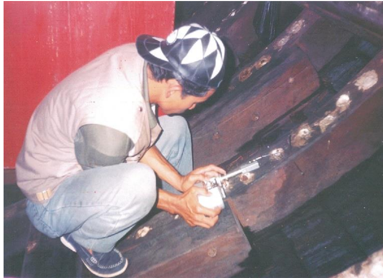
Fig. 7 Vibration measurement using a handvibrograph
