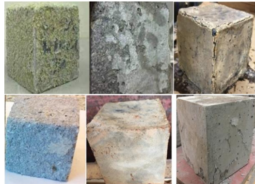
Fig. 9 Deteriorated bacterial concrete cubes taken out from \text{Na}_2 \text{SO}_4 solution after 365 days
