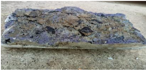
Fig. 6 Specimens prepared for seawater immersion for bulk diffusion test
