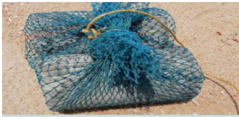
Fig. 6 Specimens prepared for seawater immersion for bulk diffusion test
