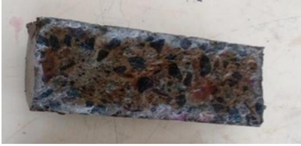
Fig. 5 White precipitate after the application of AgNO 3
