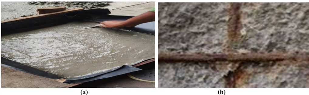
Fig. 12 (a) Normal concrete slabs during casting, and (b) Corroded bars in normal concrete slabs.
