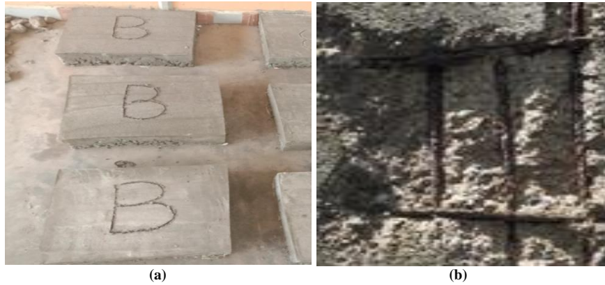
Fig. 13 (a) Bacterial concrete slabs before immersion in seawater, and (b) Corroded bars in bacterial concrete slabs.
