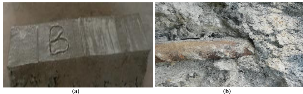
Fig. 11 (a) Bacterial concrete beams before immersion in seawater, and (b) Corroded bars in bacterial concrete beams.
