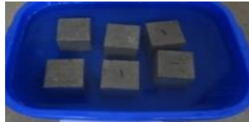
Fig. 8 Cubes immersed in 5% \text{Na}_2\text{SO}_4 solution for 365 days
