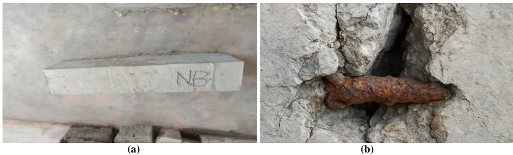
Fig. 10 (a) Normal concrete beams before immersion in seawater, and (b) Corroded bars in normal concrete beams.
