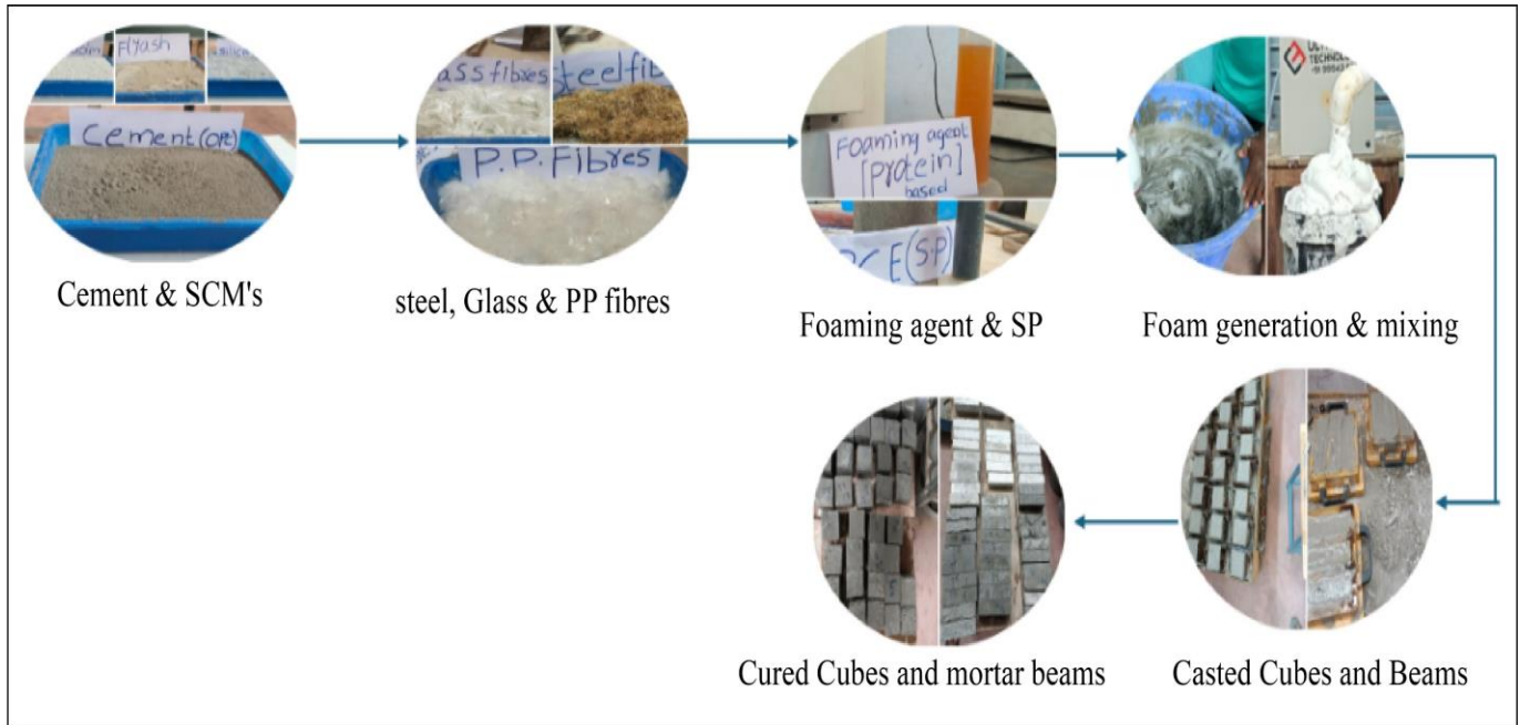
Fig. 2 Experimental workflow for the fibre reinforced foam cement mix
