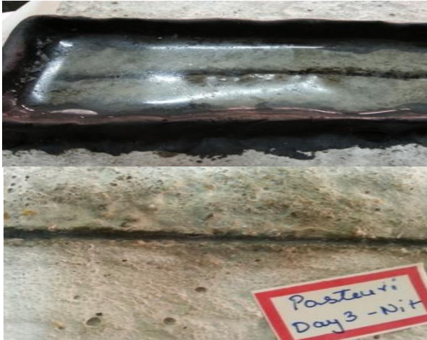
Fig. 7 Ponding and Injection Technique used for Crack Healing
