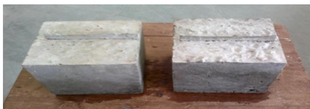
Fig. 6 An Aluminum sheet was used to simulate an unhealed crack
