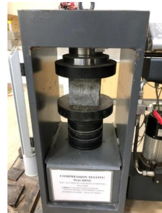
Fig. 9 Cube testing in CTM
