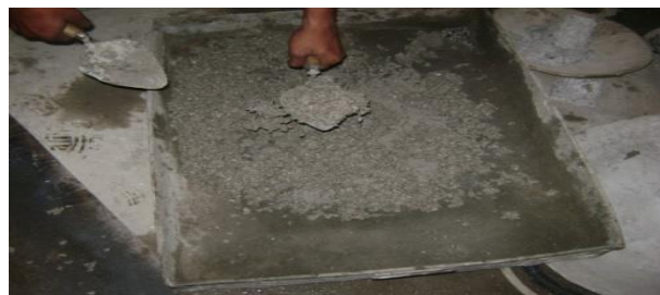
Fig. 4 Concrete being poured into a tray from a pan mixer
