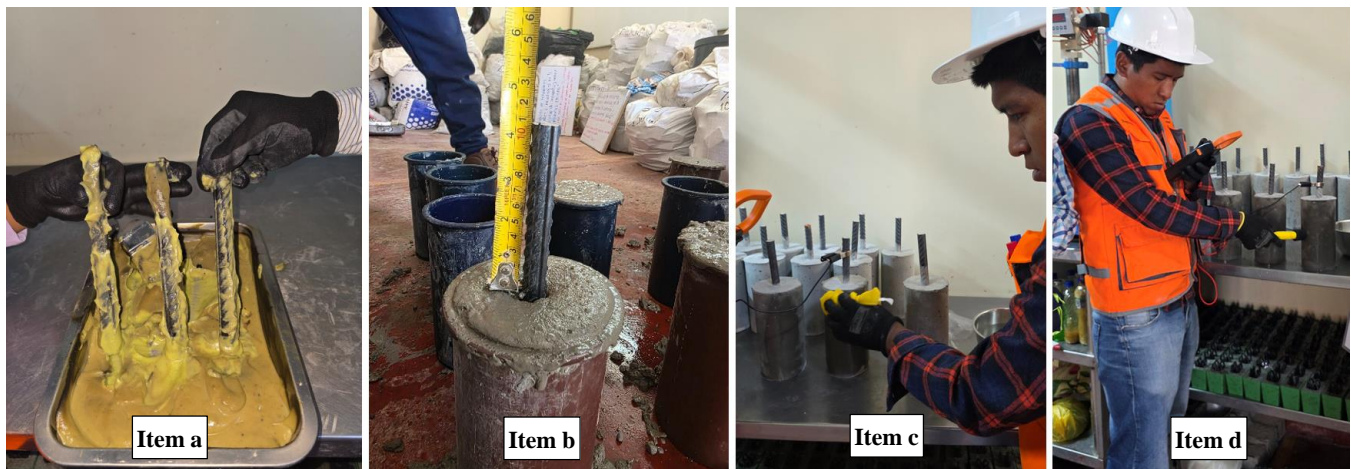
Fig. 13 ASTM C876 test procedure
