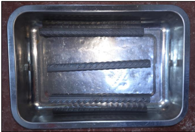
Fig. 4 ASTM A615 Grade 60 5/8" corrugated iron
