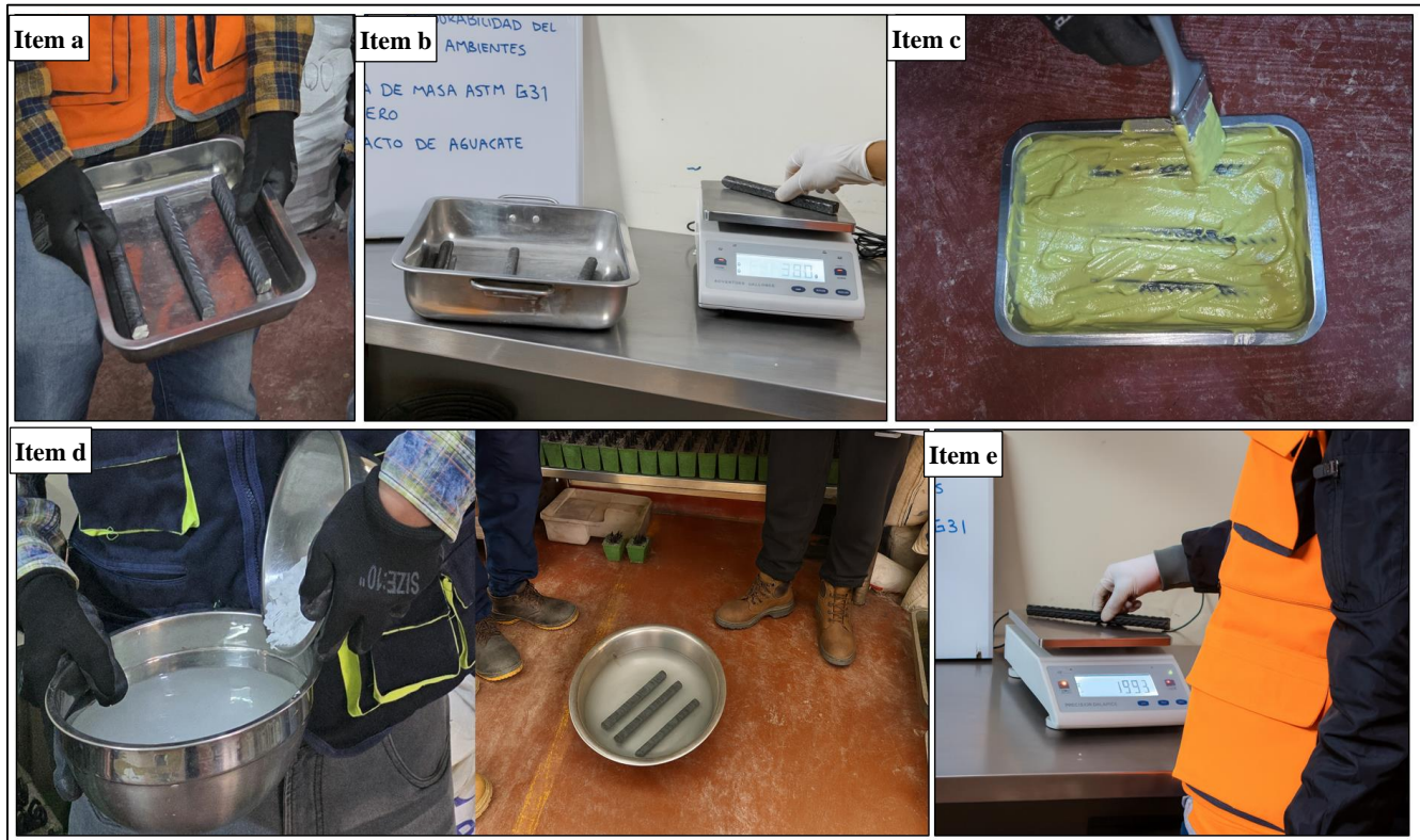
Fig. 11 ASTM G31 test procedure
