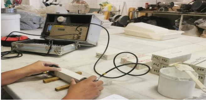
Fig. 4 Ultrasonic testing (UPV) for measuring the resistance of concrete specimens
