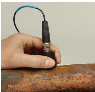
Fig. 6 Ultrasonic test (UPV-27 MG meter adaptation) to measure the resistance of steel samples
