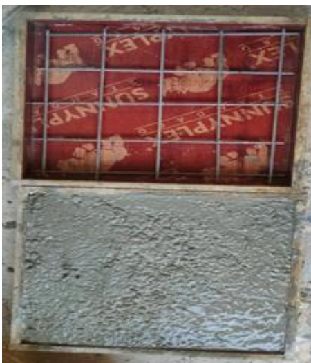
Fig. 2 Samples of the mold with reinforcement and concrete casting
