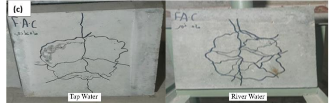
Fig. 10 Modes of failure of (a) NC, (b) SCC, and (c) FAC.
