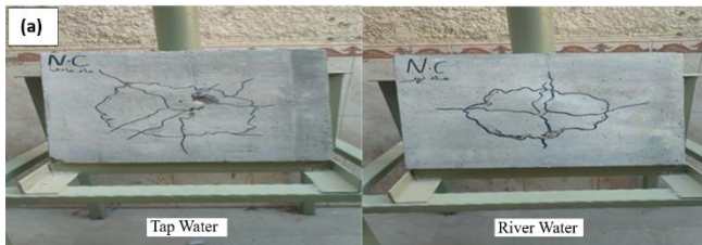
Fig. 9 Crack width of each type of concrete slab
