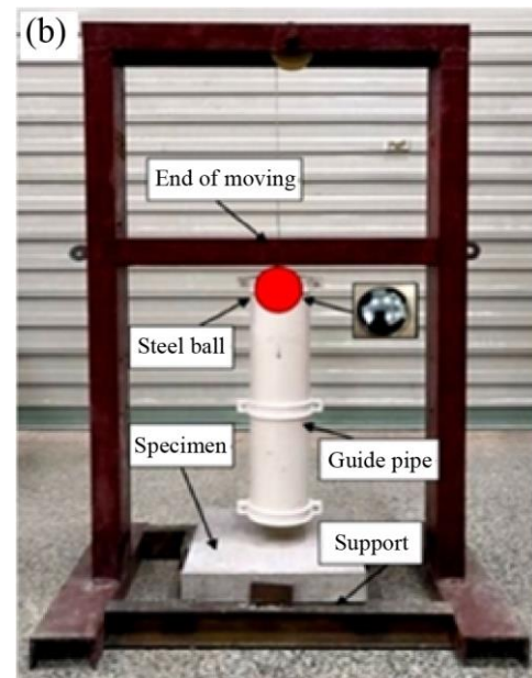
Fig. 3 Drop ball test machine (a) Used in this study, and (b) Reported in the literature [10].
